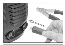
Welding rod holder lead to the (+) Positive terminal
